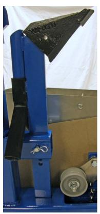
STEP 4: Attach the hitch assembly to the front of the Seeder
