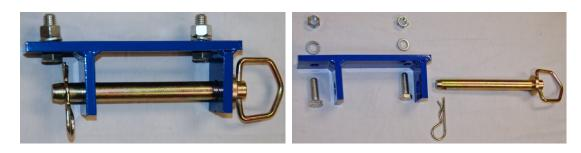
**Note**: For **Italian 2WTs**, use Hitch Adapter Assembly (Italian) 2WT (PN 601053-000). Mount the adapter assembly onto the Italian 2WT (per instructions included with the Adapter Assembly). The hitch assembly provided with the CA-Seeder 1000 will easily connect to the Adapter Assembly.
