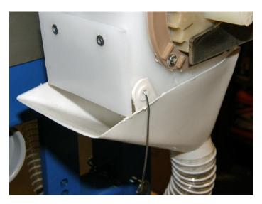
**STEP 9**: Install the fertilizer meter funnel.
